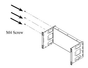
Step 3 Install Bottom Cover Panel. Place cover panel with flange facing up and short depth side cut facing forward as in illustration. Secure side brackets with (3) M4 screws to right and left side of cover panel but do not tighten them yet.
