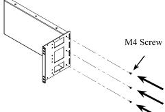
Step 2 Install Left Side Bracket. Secure side bracket with (3) M4 screws to solid panel but do not tighten them yet.
